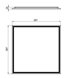
Dimensions: 597 x 597 x 25 mm Total power: 45 w Luminaire luminous flux: 4500 lm Luminaire efficacy: 100 lm/w Weight: 2.5 kg
