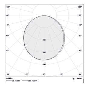
Correlated color temperature: 3000 – 6000 kelvin Rated median useful life: 50000h L70 at 25°C Luminaire input power: 45 w
