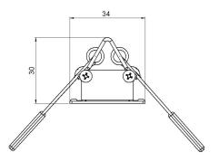
Dimensions: 1000 x 34 x 30 mm Total power: 15 w Luminaire luminous flux: 1500 lm Luminaire efficacy: 100 lm/w Weight: 0.6 kg
