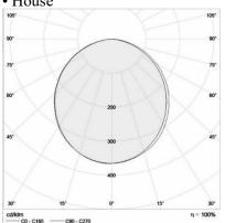
Correlated color temperature: 3000 – 6000 kelvin Rated median useful life: 50000h L70 at 25°C Luminaire Luminaire input power: 15 w/m
