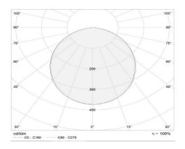
Correlated color temperature: 3000-4000-6000 kelvin Rated median useful life: 50000h L70 at 25°C Luminaire input power: 90w
