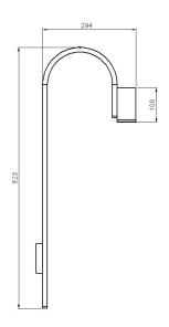
Dimensions: 294 x 823 mm Total power: 15 w Luminaire luminous flux: 1650 lm Luminaire efficacy: 110 lm/w Weight: 3 kg
