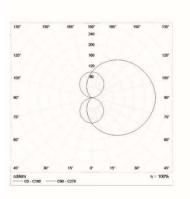
Correlated color temperature: 3000-6000 kelvin Rated median useful life: 50000h L70 at 25°C Luminaire input power: 15 w
