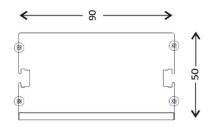
Dimensions: 1000 x 90 x 50 mm Total power: 30 w Luminaire luminous flux: 3000 lm Luminaire efficacy: 100 lm/w Weight: 1.8 kg
