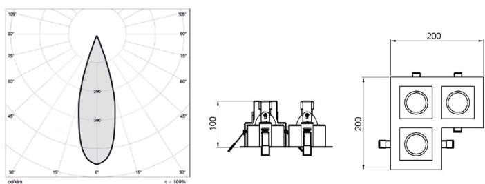
Correlated color temperature: 3000 – 6000 kelvin Rated median useful life: 50000h L70 at 25°C Luminaire input power: 3 x 7 w Dimensions: 200 x 200 x 100 mm Total power: 3 x GU10 (7w) Weight: 1.4 kg
