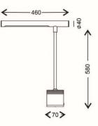
Dimensions: Ø40 x 70 x 580 mm Total power: 9 W Luminaire luminous flux: 540 lm Luminaire efficacy: 60 lm/w Weight: 4 kg
